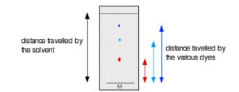
The R<sub>f</sub> value for each dye is then worked out using the formula:
