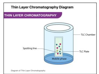
If working with an ink on paper. First extract the ink sample from the paper. Using a capillary tube, wick up an ink sample. Apply capillary tube to starting line on the TLC paper to create a spot. Duly note on the TLC paper which sample is applied. If working with dilute samples we can achieve better results by drying the application and re-applying. Repeat until applied 3-5 times.
